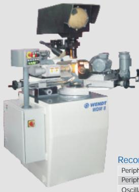
Peripheral speed of the Hybrid Grinding Wheel: 3 – 5 m/sec. Peripheral speed of the Al<sub>2</sub>O<sub>3</sub>Wheel: 15 - 28 m/sec. Oscillation speed: 200 - 1000 mm/min. In feed: 0.01 – 0.07 mm per stroke
